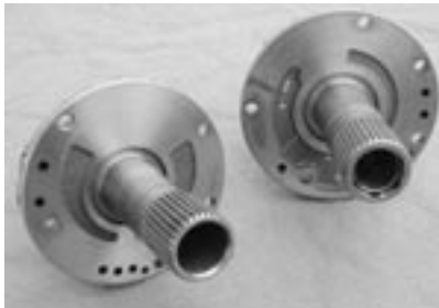
The AODE's stock pump stator is on the right. To improve lubrication and cooling flow, Lentech modifies AOD stators for use in the AODE Strip Terminator.
