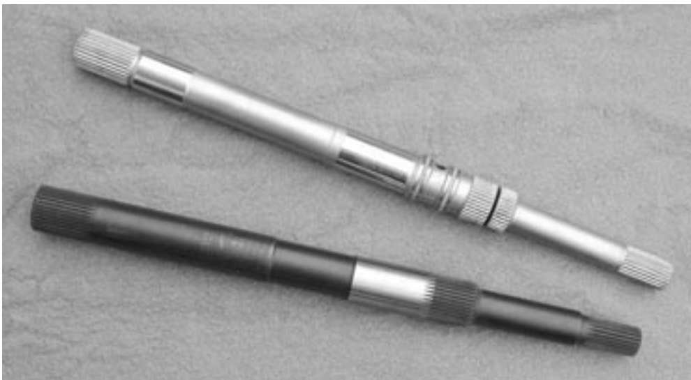
The AODE's stock pump stator is on the right. To improve lubrication and cooling flow, Lentech modifies AOD stators for use in the AODE Strip Terminator.
