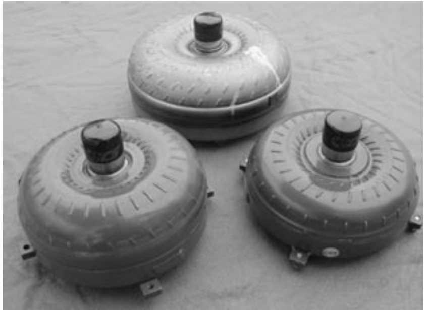
A factory 12-inch, clutch-equipped AODE converter (about 51 pounds) is shown at the rear, an aftermarket clutch-equipped 10-incher (31.5 pounds) is on the left, and a 10-inch nonclutched version (26 pounds) as fitted to the AODE Strip Terminator is on the right. Going with a nonlockup converter greatly decreases rotating mass, for better response and acceleration, as well as eliminates the strength limitations of a lockup clutch.
